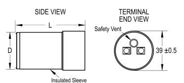
General Information Series MS/A902 Dielectric Aluminum Electrolytic Description Motor Start Aluminum Electrolytic RoHS Lead **Quick Connect** AEC-Q200 No Halogen Free Yes Shelf Life 156 Weeks
