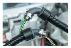
External Metric thread provides a secure connection. Snap-on construction reduces installation time and costs by eliminating the need to thread fittings onto conduits.
