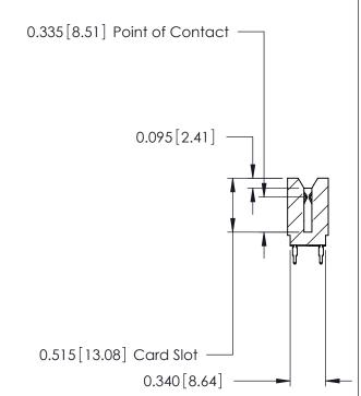
746 Series Ultra-Mate Card Edge Connector - Press Fit Part Number: 746-058-525-206
