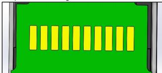
The current PCBs feature solder mask on the nonsolderable Gold surface pads on the bottom of the PCB.
