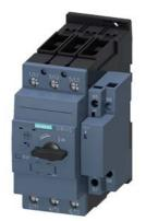
Circuit breaker size S2 for motor protection, CLASS 10 with overload relay function A-release 28...36 A N-release 520 A Standard switching capacity
