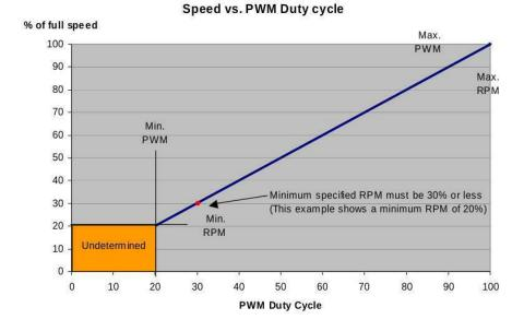
This can vary from fan to fan. Ideally, this information will be given in a fan's datasheet. For example, this if from the datasheet for a Delta Electronics AUB0912VH fan:
