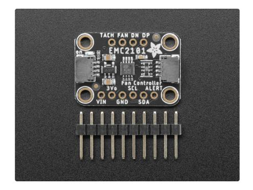
Four pin PC fans have a power and ground pin (those are often red and black) and then two more pins. One of those extra pins, the PWM pin, allows you to set a the speed of the fan. The last TACH pin is for a tachometer output that allows the EMC2101 to monitor the speed of the fan to make sure it's working as expected. Instead of using an PWM output and counter input on your microcontroller, this chip will take care of that all for you, all over every-day I2C.
