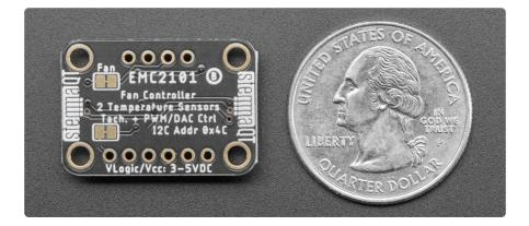
This neat little chip can easily be used to help provide cooling or ventilation to your next project. You might even be able to use it to help quiet down an existing project or hack a noisy piece of electronics that has a loud fan. By allowing you to run a fan at
