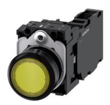
Illuminated pushbutton, 22 mm, round, plastic, yellow, pushbutton, flat, momentary contact type, with holder, 1 NO+1 NC, LED module with integrated LED 110 V AC, screw terminal, with laser labeling, lower case
