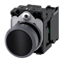
Pushbutton, 22 mm, round, plastic with metal front ring, black, pushbutton, flat, momentary contact type, with holder, 1 NO, screw terminal, with laser labeling, upper case
