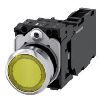
Illuminated pushbutton, 22 mm, round, Metal, shiny, yellow, pushbutton, flat, momentary contact type, with holder, 1 NO+1 NC, LED module with integrated LED 230 V AC, screw terminal, with laser labeling, lower case
