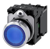
Illuminated pushbutton, 22 mm, round, Metal, shiny, blue, pushbutton, flat, momentary contact type, with holder, 1NO, LED module with integrated LED 230 V AC, screw terminal, with laser labeling, inscription or symbol Customer-specific selection with SIRIUS ACT configurator (CIN)
