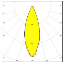
Dimensions: 69.5 mm x 69.5 mm Height: 41.50 mm ~35° medium beam. Assembly with holder C compatible with LEDiL HEKLA.
