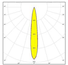
Dimensions: 69.5 mm x 69.5 mm Height: 41.50 mm ~14° spot beam. Assembly with holder C compatible with LEDiL HEKLA.
