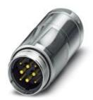
Coupler connector, straight, for standard and SPEEDCON interlock, M40, number of positions: 4+3+PE, type of contact: Pin, Crimp connection, shielded: yes, cable diameter range: 20.5 mm ... 26.5 mm
