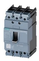
circuit breaker 3VA5 UL frame 125 breaking capacity class S 25kA @ 480 V 3-pole, line protection TM210, FTFM, In=110A overload protection Ir=110A fixed short-circuit protection li=10 x In UL489 SB (naval), 50 deg. cel. cable connection on both sides
