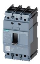
circuit breaker 3VA5 UL frame 125 breaking capacity class M 35kA @ 480 V 3-pole, line protection TM210, FTFM, In=30A overload protection Ir=30A fixed short-circuit protection Ii=10 x In UL489 SB (naval), 50 deg. cel. cable connection on both sides
