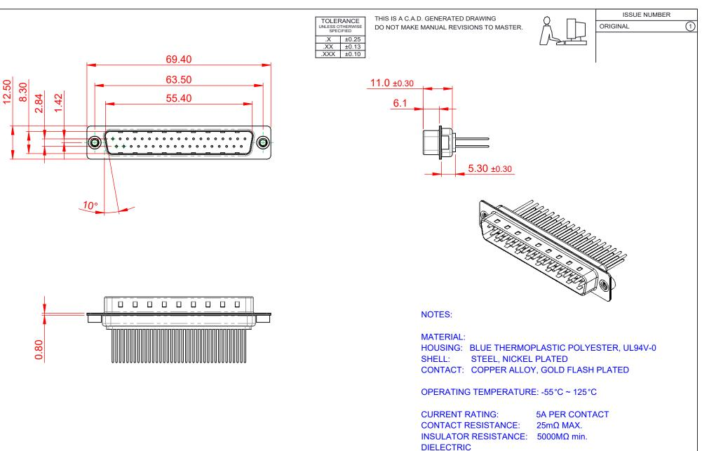
WITHSTANDING VOLTAGE: 1000V AC rms
