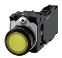
Illuminated pushbutton, 22 mm, round, plastic, yellow, pushbutton, flat, momentary contact type, with holder, 1 NO+1 NC, LED module with integrated LED 110 V AC, screw terminal, with laser labeling, upper case
