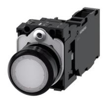
Illuminated pushbutton, 22 mm, round, plastic, white, pushbutton, flat, momentary contact type, with holder, 1 NO+1 NC, LED module with integrated LED 110 V AC, screw terminal, with laser labeling, upper case
