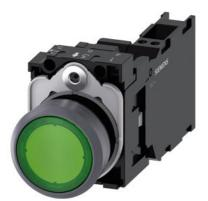
Illuminated pushbutton, 22 mm, round, plastic with metal front ring, green, pushbutton, flat, momentary contact type, with holder, 1 NO+1 NC, LED module with integrated LED 24 V AC/DC, spring-type terminal, with laser labeling, inscription or symbol Customer-specific selection with SIRIUS ACT configurator (CIN)
