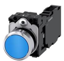
Pushbutton, 22 mm, round, metal, shiny, blue, pushbutton, flat, momentary contact type, 1 NO+1 NC, screw terminal, with laser labeling, lower case
