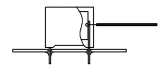
Temperature monitored inside the capacitor.
