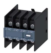
Auxiliary switch on the front, 4 NO Current path 1 NO, 1 NO, 1 NO, 1 NO for 3RH and 3RT Ring cable lug connection .3/.4, .3/.4, .3/.4, .3/.4
