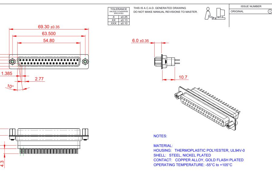
CURRENT RATING: 3A PER CONTACT CONTACT RESISTANCE: 25mQ MAX. INSULATOR RESISTANCE: 5000MΩ min. DIELECTRIC WITHSTANDING VOLTAGE: 1000V AC rms
