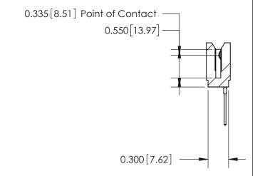
745 Series Ultra-Mate Card Edge Connector - Press Fit ACAD REFERENCE NO. Part Number: 745-043-545-106
