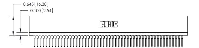
745 Series Ultra-Mate Card Edge Connector - Press Fit
