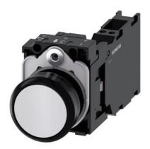
Pushbutton, 22 mm, round, plastic, white, pushbutton, flat, momentary contact type, with holder 1 NO+1 NC, spring-type terminal, Z=20-unit packaging
