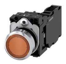
Illuminated pushbutton, 22 mm, round, metal, shiny, amber, pushbutton, flat, momentary contact type, with holder, 1 NO+1 NC, LED module with integrated LED 110 V AC, screw terminal, with laser labeling, inscription or symbol Customer-specific selection with SIRIUS ACT configurator (CIN)
