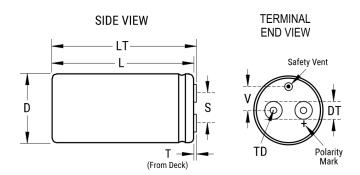
General Information Series ALS30 Dielectric Aluminum Electrolytic Description Screw Terminal, Aluminum Electrolytic RoHS AEC-Q200 No Component 690 g Weight Dimensions D And L Include Sleeving. MS (MxH) = Notes M12x16. Mounting Clamp (Sold Separately): V11 Shelf Life 156 Weeks
