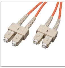
**Description**Tripp Lite's 3-ft. (0.91 m) multimode duplex fiber optic SC/SC patch cable is manufactured from 62.5/125 zipcord fiber. The cable has SC connectors on each end, a PVC jacket and is FDDI and OFNR rated. duplex multimode fiber is most commonly used in LAN applications.
