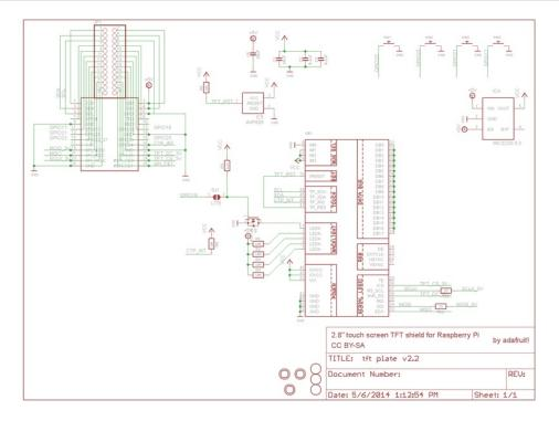
Schematic for PiTFT Plus (B+/Pi 2 shape)
