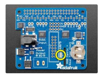
If you're using a 64x64 RGB matrix and either a Bonnet or a Rev C HAT, use your soldering iron to melt a blob of solder on the bottom solder jumper so the middle pad is 'shorted' to 8. (This is compatible with 64x64 matrices in the Adafruit store. For 64x64 matrices from other sources, you might need to use 16 instead, check the datasheet.)
