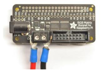
Plug the red wire into the + side, and the black wire into the - side.
