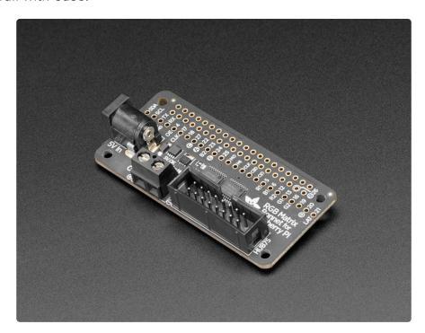
"Bonnet" boards work on any Raspberry Pi with a 40-pin GPIO header — Zero, Zero W/WH, Model A+, B+, Pi 2, 3 and 4. They do not work with older 26-pin boards like the
