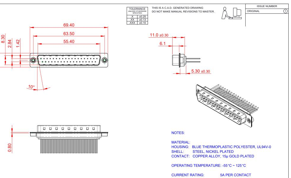
CONTACT RESISTANCE:  $25m\Omega$  MAX. INSULATOR RESISTANCE: 5000MΩ min. DIELECTRIC WITHSTANDING VOLTAGE: 1000V AC rms
