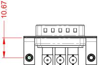
75Ω (IMPEDANCE) **POWER/CO-AX CONTACT RATING:** (IF PRESENT) SIGNAL CONTACT CURRENT RATING: 5A PER CONTACT SIGNAL CONTACT RESISTANCE:  $10m\Omega$  MAX.
