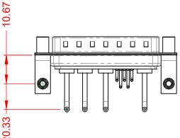
POWER/CO-AX CONTACT RATING: (IF PRESENT) SIGNAL CONTACT CURRENT RATING: 5A PER CONTACT SIGNAL CONTACT RESISTANCE:  $10m\Omega$  MAX.
