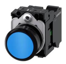
Pushbutton, 22 mm, round, plastic, blue, pushbutton, flat, momentary contact type, with holder 1 NO, spring-type terminal, with laser labeling, symbol number according to, ISO 7000 or IEC 60417
