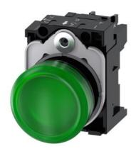
Indicator lights, 22 mm, round, plastic, green, lens, smooth, with holder, LED module with integrated LED 110 V AC, screw terminal, with laser labeling, symbol number according to, ISO 7000 or IEC 60417
