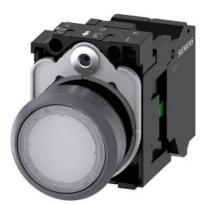
Illuminated pushbutton, 22 mm, round, plastic with metal front ring, white, pushbutton, flat, momentary contact type, with holder, 1NO, LED module with integrated LED 24 V AC/DC, spring-type terminal, with laser labeling, upper case
