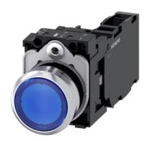
Illuminated pushbutton, 22 mm, round, metal, shiny, blue, pushbutton, flat, momentary contact type, with holder, 1 NO+1 NC, LED module with integrated LED 110 V AC, screw terminal, with laser labeling, lower case
