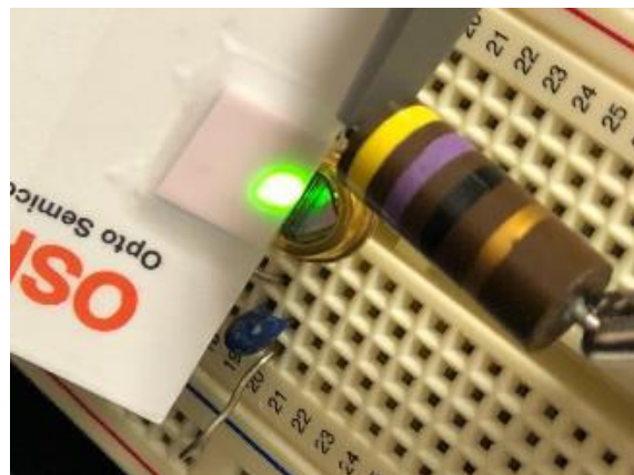
Figure 6: The sensor should be placed in the focused laser beam region.
