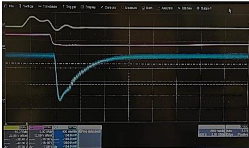
Fig. 3: The frequency generator (yellow/top trace) is shown from frequency generator/J5 while the current pulse which is pulsed across the laser shown in the pink/middle trace (J7). The bottom trace which is discussed later, is the output of a detector.
