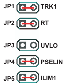
Figure 7. Configure the EVM as a Slave for Stackable Operation
