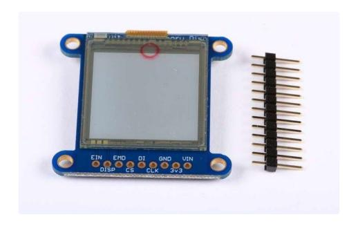
The display and support circuitry come pre-assembled and fully tested on a handy breakout board. For use in a breadboard, you will want to install the included 0.1" header strip:
