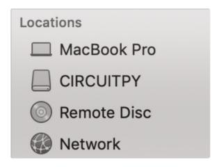
After it finished uploading, and with the Circuit Playground board connected over USB, it should appear on your computer as a flash drive called **CIRCUITPY**.
