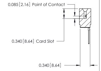
ACAD REFERENCE NO. 746 Series Ultra-Mate Card Edge Connector - Press Fit DRAWN: Part Number: 746-034-540-501 CHECKED: **EDAC INC** THESE DRAWINGS AND SPECIFICATIONS ARE THE PROPERTY OF EDAC INC., AND TORONTO, ONTARIO SHALL NOT BE REPRODUCED, OR COPIED CANADA OR USED AS THE BASIS FOR THE MANUFACTURE OR SALE OF APPARATUS
