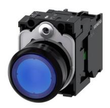
Illuminated pushbutton, 22 mm, round, plastic, blue, pushbutton, flat, momentary contact type, with holder, 1NO, LED module with integrated LED 24 V AC/DC, screw terminal, with laser labeling, upper case
