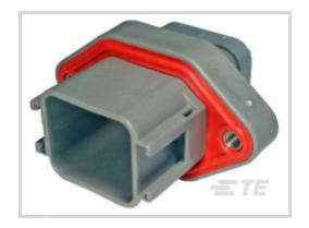
Connector & Housing Type: Housing for Male Terminals Mating Pin Diameter: 1.59 mm [.063 in ] Connector System: Wire-to-Wire Number of Positions: 18
