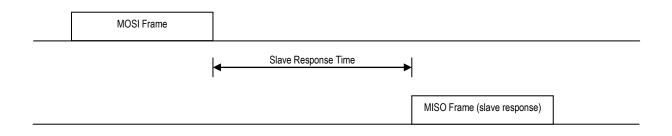
The timeout should be at least **2** \* **'Slave Response Time max'** and in none real time systems it should not be smaller than **200ms** due to possible system side delays.
