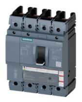
circuit breaker 3VA5 UL frame 250 breaking capacity class M 35kA @ 480 V 4-pole, line protection TM230, FTAM, In=110A overload protection Ir=110A fixed short-circuit protection Ii=5...10 x In N conductor protection 100% without connection
