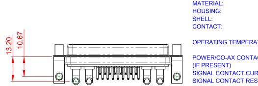
THERMOPLASTIC POLYESTER, UL94V-0 STEEL, NICKEL PLATED COPPER ALLOY, 30µ GOLD PLATED
