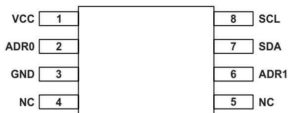
Package LE, 8-Pin TSSOP Pinout Diagram
