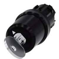
key-operated switch Siemens, 22 mm, round, plastic, lock number SSG10, with 2 keys, 2 switch positions O<I, momentary contact type, actuating angle 45°, 10:30h/12h, key removal O, with laser labeling, upper case and lower case, always upper case at the beginning of the word
