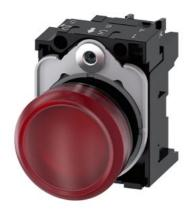
Indicator lights, 22 mm, round, plastic, red, lens, smooth, with holder, LED module, with integrated LED 230 V AC, screw terminal, with laser labeling, symbol number according to, ISO 7000 or IEC 60417
