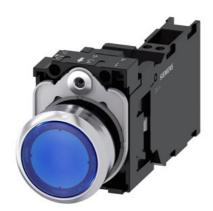
Illuminated pushbutton, 22 mm, round, Metal, shiny, blue, pushbutton, flat, momentary contact type, with holder, 1 NO+1 NC, LED module with integrated LED 230 V AC, spring-type terminal, with laser labeling, symbol number according to, ISO 7000 or IEC 60417
